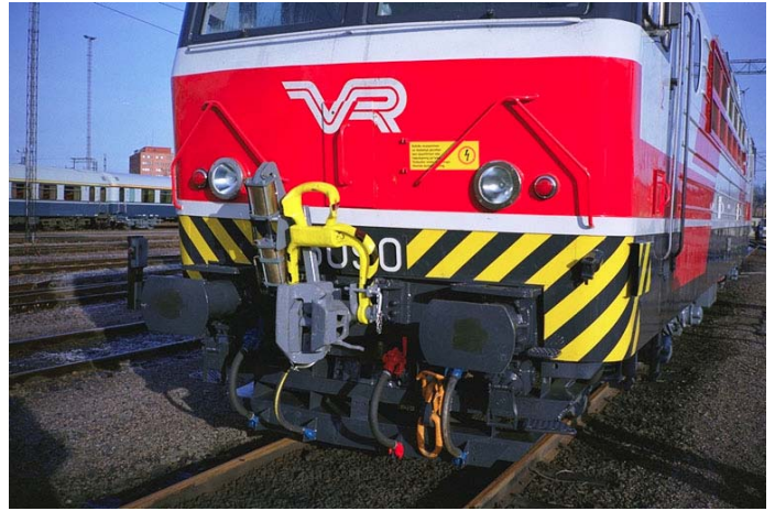
Fig. 3. Finnish locomotive fitted with both European and Russian couplers and buffers.
