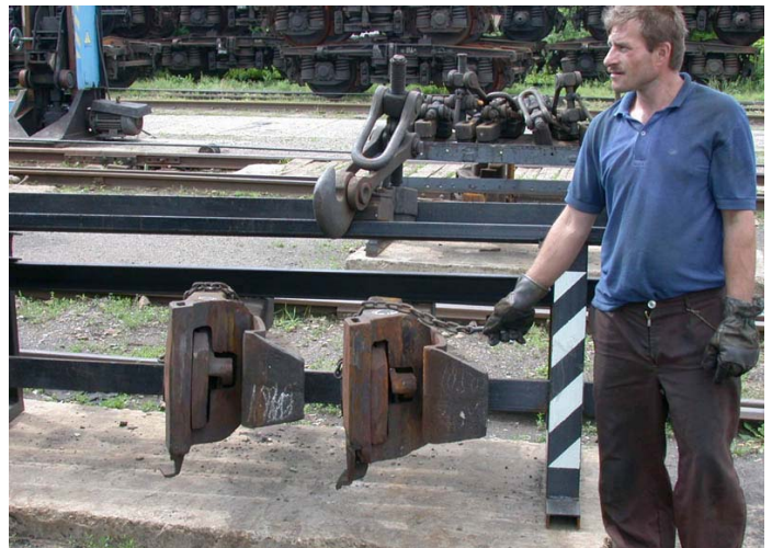
Fig. 4. European screw-link and Russian SA3 automatic couplers at a transfer station on the Polish-Ukrainian border.
