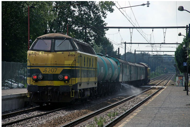
Picture of Month Detail: Belgian SNCB weed killing train, at Limal near Ottignies.
