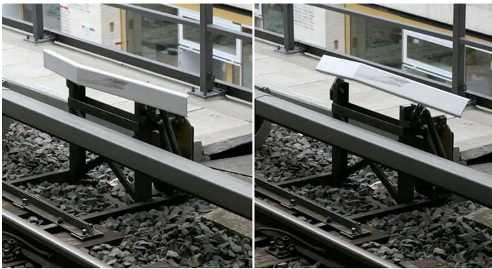
Left: Red signal, the white bar touches a valve which stops the train. Right: The white bar is tilted away.
